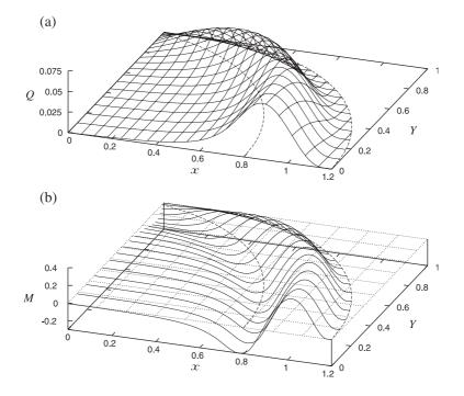
Fig. 12. Analytical solutions for (a) net flux Q over a period; (b) net deposition  $M = -\partial Q/\partial x$  over a period under axial flow, for case (iv) with n=1. Dashed lines indicate the positions of the shoreline at maximum run-up and run-down; dotted grid indicates the surface M=0 (no net erosion or deposition). The maximum bed level change in dimensional variables is  $|\hat{Z}_e| \approx 5.4$  cm over an hour of seiching.
