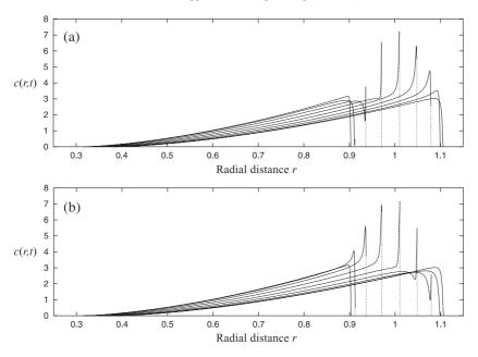
Fig. 15. Analytical solution for suspended sediment concentration under radial flow, for case (i) with n = 1. (a) Outward flow; (b) inward flow.
