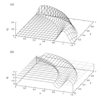
Fig. 7. Analytical solutions for (a) net flux Q over a period; (b) net deposition  $M = -\partial Q/\partial x$  over a period under axial flow, for reference case (i) with n = 3. Dashed lines indicate the positions of the shoreline at maximum run-up and run-down; dotted grid indicates the surface M = 0 (no net erosion or deposition). The maximum bed level change in dimensional variables is  $|\hat{Z}_e| \approx 1.3$  cm over an hour of seiching.
