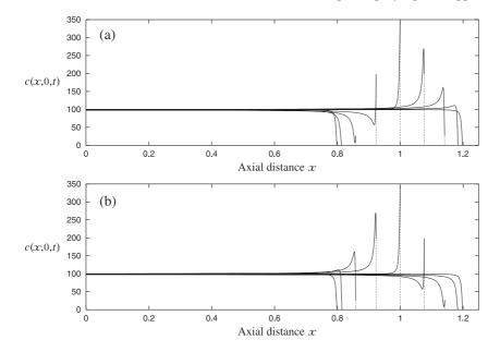
Fig. 6. Analytical solution for suspended sediment concentration under axial flow, for reference case (i) with n=3. (a) On-shore flow; (b) offshore flow.
