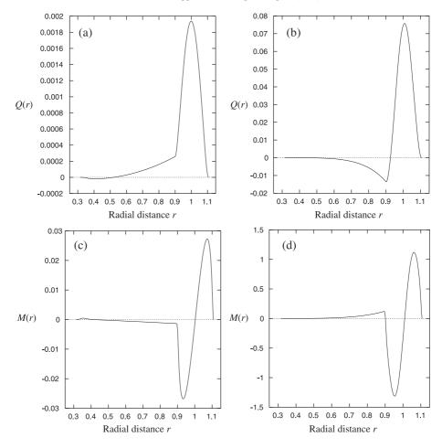
Fig. 17. Residual net sediment flux Q(r) and net deposition M(r) under radial seiching flow, for case (i) with n = 1 (a, c) and for n = 3 (b, d). The maximum bed level change for n = 1 is  $|\hat{Z}_e| \approx 8$  mm, and for n = 3 is  $|\hat{Z}_e| \approx 1.3$  cm, each over 1 hour.
