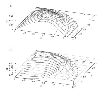
Fig. 11. Analytical solutions for (a) net flux Q over a period; (b) net deposition  $M = -\partial Q/\partial x$  over a period under axial flow, for case (ii) with n = 1. Dashed lines indicate the positions of the shoreline at maximum run-up and run-down; dotted grid indicates the surface M = 0 (no net erosion or deposition). The maximum bed level change in dimensional variables is  $|\hat{Z}_e| \approx 1.6$  cm over an hour of seiching.
