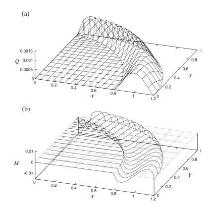
Fig. 9. Analytical solutions for (a) net flux Q over a period; (b) net deposition  $M = -\partial Q/\partial x$  over a period under axial flow, for case (iii) with n=1. Dashed lines indicate the positions of the shoreline at maximum run-up and run-down; dotted grid indicates the surface M=0 (no net erosion or deposition). The maximum bed level change in dimensional variables is  $|\hat{Z}_e| \approx 1.3$  mm over an hour of seiching.
