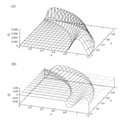
Fig. 5. Analytical solutions for (a) net flux Q over a period; (b) net deposition  $M = -\partial Q/\partial x$  over a period under axial flow, for reference case (i) with n = 1. Dashed lines indicate the positions of the shoreline at maximum run-up and run-down; dotted grid indicates the surface M = 0 (no net erosion or deposition).
