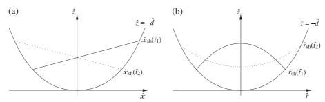
Fig. 1. Schematics (vertical scale exaggerated) showing cross sections of the basin with surface elevations at two points of the oscillation (solid and dotted lines): (a) axial mode (Section 3); (b) radial mode (Section 4).
