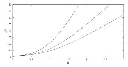
Fig. 2. The ratio between near-bed and depth-averaged sediment concentrations for various values of the Rouse number  $B_0$  and for  $\eta_b = 0.01$  (top line), 0.02, 0.03 (bottom line).
