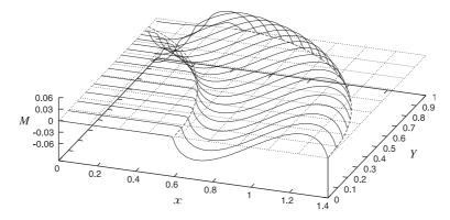
Fig. 8. Analytical solution net deposition  $M = -\partial Q/\partial x$  over a period under axial flow, for reference case (i) with n = 1 and the revised values A = 0.4,  $u_e = 0.2$ . Dashed lines indicate the positions of the shoreline at maximum run-up and run-down; dotted grid indicates the surface M = 0 (no net erosion or deposition). The maximum bed level change in dimensional variables is  $|\hat{Z}_e| \approx 8$  mm over an hour of seiching.
