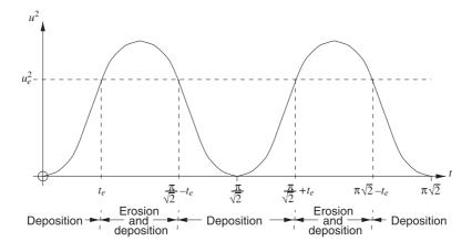
Fig. 3. Schematic illustrating the magnitude of  $u^2$  as a function of time, and the corresponding intervals of simultaneous erosion/deposition and of pure deposition. These are used to construct the Lagrangian concentration field.
