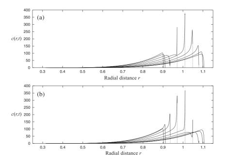
Fig. 16. Analytical solution for suspended sediment concentration under radial flow, for case (i) with n=3. (a) Outward flow; (b) inward flow.
