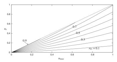
Fig. 13. Selected contours of  $r_{0*}(u_{\text{max}}, u_e)$  (solid lines), together with the boundary  $u_e = u_{\text{max}}$  of the regime in which sediment can be mobilised (dashed line). Lowest line represents  $r_{0*} = 0.1$ , uppermost represents  $r_{0*} = 0.9$ .
