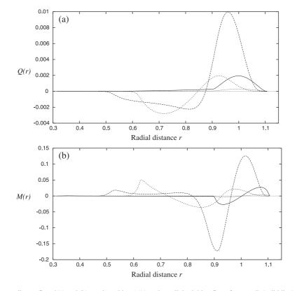
Fig. 18. (a) Residual net sediment flux Q(r) and (b) net deposition M(r) under radial seiching flow, for case (i) (solid line); case (ii) (light dashed line); case (iii) (dotted line); case (iv) (heavy dashed line). The exponent n = 1 in each case.
