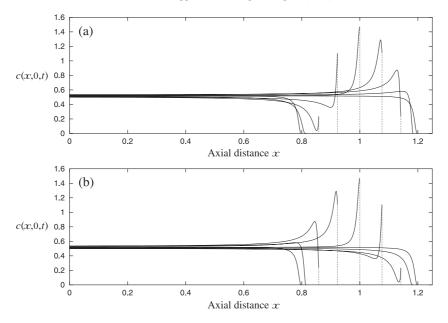
Fig. 10. Analytical solution for suspended sediment concentration under axial flow, for case (ii) with n = 1. (a) On-shore flow; (b) off-shore flow.
