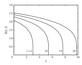
FIGURE 22. The scaled height of the current as a function of downslope distance at various instances of time from the similarity solution for unsteady propagation along a horizontal channel.
