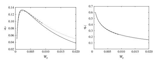
FIGURE 6. The dimensionless volume flux per unit width transported by the flowing layer,  $\hat{q}$ , and the depth-averaged volume fraction,  $\phi$ , as functions of the dimensionless strength of the fluidising gas flow,  $W_g$ , for parameter values  $R = 10^{-3}$ ,  $\psi = 0.50$ ,  $\phi_m = 0.63$ , e = 0.85,  $e_w = 0.75$ , S = 0.10, St = 0.10 and  $\delta = 10^{-2}$ . Also plotted are the asymptotic solutions (dashed) and the simple approximate solutions (dotted).
