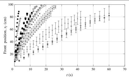
FIGURE 20. The position of the front of the fluidised current as a function of time for varying source fluxes and fluidising gas flows.
