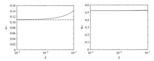
FIGURE 5. The dimensionless volume flux per unit width transported by the flowing layer,  $\hat{q}$ , and the depth-averaged volume fraction,  $\bar{\phi}$ , as functions of the relative particle size for parameter values  $R = 10^{-3}$ ,  $\psi = 0.50$ ,  $\phi_m = 0.63$ , e = 0.85,  $e_w = 0.75$ , S = 0.10, St = 0.10 $10^3 \delta^2$  and  $W_g = 10^{-3}$ . Also plotted are the asymptotic solutions (dashed) and the simple approximate solutions (dotted).
