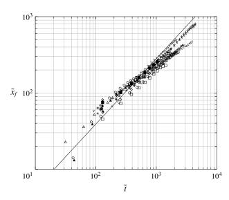
FIGURE 23. The scaled position of the front of the current,  $\tilde{x}_f$  as a function of scaled time. The data are drawn from figure 20 with distance and time scales according to (5.4) and theoretical line given by (6.10) (solid line). Key is as per figure 20.
