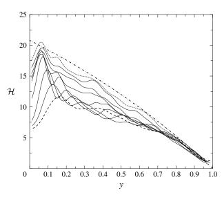
FIGURE 27. The scaled depth of the fluidised current along a horizontal channel,  $\mathcal{H}$ , as a function of the scaled position,  $y = \bar{x}/\bar{x}_f$ . The data are drawn from figure 21 scaled using (5.4). The model solution is from (6.29) and is represented by the chain-dotted line.
