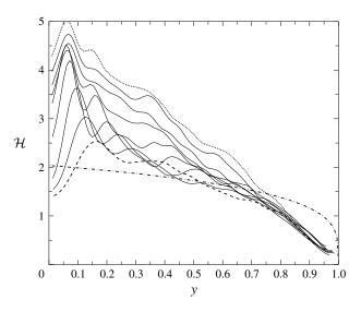
FIGURE 24. The scaled height of the current,  $\mathcal{H}$ , as a function of the scaled distance,  $y = \tilde{x}/\tilde{x}_f$ , at various instants of time. The data are drawn from figure 21 scaled using (6.10). The model solution (6.10) is represented by the chain-dotted line.
