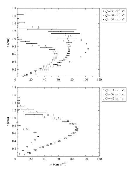
FIGURE 11. Ensemble-averaged velocity profiles for steady flows for  $\theta = 10^{\circ}$  and  $\theta = 15^{\circ}$ . Error bars are 95 % confidence limits calculated from (2.2) with m = 5 and n = 16.
