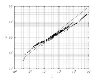
FIGURE 26. The scaled position of the front of the fluidised current in a horizontal channel as a function time. The data are those plotted in figure 20 and scaled using (6.25)with the model prediction from (6.30) (solid line). The key is given in figure 20.
