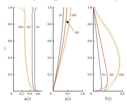
FIGURE 4. (Colour online) The volume fraction,  $\phi(\hat{z})$ , velocity of the solid phase,  $\hat{v}(\hat{z})$ , and the granular temperature,  $\hat{T}(\hat{z})$ , as functions of the dimensionless depth within the current for parameter values  $R = 10^{-3}$ ,  $\psi = 0.3$ ,  $\phi_m = 0.63$ , e = 0.85,  $e_w = 0.75$ , St = 0.750.1,  $\delta = 0.01$ ,  $W_g = 10^{-3}$ , (i) S = 0.1; (ii) S = 0.2 and (iii) S = 0.3. Also plotted are the asymptotic solutions (dotted lines).
