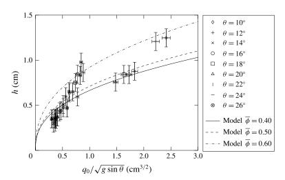
FIGURE 10. The height of the flowing layer as a function of the scaled volume flux,  $q_0/\sqrt{g\sin\theta}$ , for a range of channel inclinations. The model curves are for (4.46) with  $\phi_m = 0.63$  and e = 0.85.
