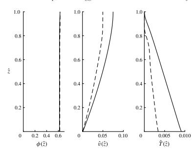
FIGURE 29. The volume fraction,  $\phi(\hat{z})$ , velocity of the solid phase,  $\hat{v}(\hat{z})$ , and the granular temperature,  $\hat{T}(\hat{z})$ , as functions of the dimensionless depth within the current for parameter values  $R = 10^{-3}$ ,  $\psi = 0.5$ ,  $\phi_m = 0.63$ , e = 0.85,  $e_w = 0.75$ , S = 0.1,  $St = 10^3 \delta^2$ ,  $\delta = 0.01$ and  $W_e = 4.1 \times 10^{-4}$  for extended kinetic theory (solid lines) and 'standard' kinetic theory (dashed lines).
