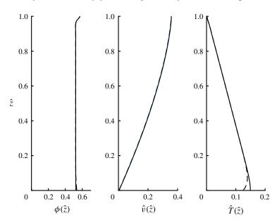
FIGURE 28. The volume fraction,  $\phi(\hat{z})$ , velocity of the solid phase,  $\hat{v}(\hat{z})$  and the granular temperature,  $\hat{T}(\hat{z})$ , as functions of the dimensionless depth within the current for parameter values  $R = 10^{-3}$ ,  $\psi = 0.5$ ,  $\phi_m = 0.63$ , e = 0.85,  $e_w = 0.75$ , S = 0.1,  $St = 10^3 \delta^2$ ,  $\delta = 0.01$  and  $W_g = 10^{-3}$  for extended kinetic theory (solid lines) and 'standard' kinetic theory (dashed lines).
