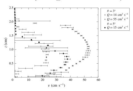
FIGURE 12. Measured velocity profiles from experiment for individual fluidised granular flows that are potentially unsteady when they are at shallow angles. Error bars are calculated from (2.1) with values of  $c_1$  determined from the correlation functions calculated during the PIV analysis.
