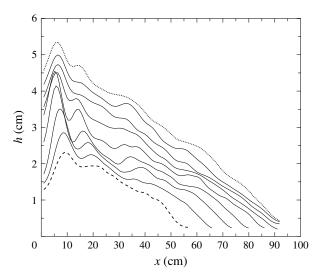
FIGURE 21. Change in shape of horizontal fluidised currents with no scaling for Q =49.05 cm<sup>3</sup> s<sup>-1</sup> and  $w_g/u_{mf} = 1.5$ . The different profiles are drawn at 0.25 s intervals. The dashed line corresponds to t=1 s and the dotted line to t=3 s.
