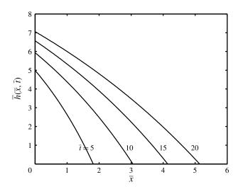
FIGURE 25. The height of the current as a function of distance along a narrow horizontal channel at various instances of time.
