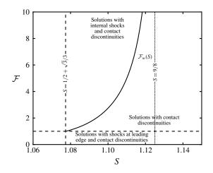
FIGURE 6. The regimes of similarity solutions in the  $(S, \mathcal{F})$  plane for  $S_f = 1$ . Also plotted is the buoyancy flux ratio at source, at which internal shocks first appear,  $\mathcal{F}_m$ , as a function of the shape factor S (solid line). The value  $S = 1/2 + \sqrt{3}/3$  is plotted (dashed line) and this corresponds to the threshold for linearly stable solutions, while solutions with internal shocks are not found for S > 9/8.
