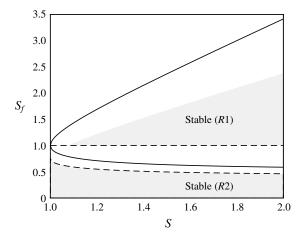
FIGURE 1. The regions R1 and R2 within the plane of shape factors,  $(S, S_f)$ , for which the steady line plume solution (2.13) is stable to harmonic disturbances to the source (shaded region, bordered by dashed lines). Also plotted are the parameter values for which the governing system of equations are ill-posed (solid lines).
