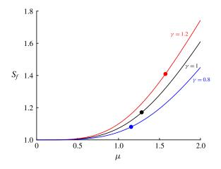
FIGURE 8. (Colour online) The shape factor,  $S_f$ , as a function of the scaled width parameter,  $\mu$ , for various ratios  $\gamma$  (see (A 25)). Also plotted are the parameter values,  $(\mu, S_f)$ , for each value of  $\gamma$  at which the line plume equations first become linearly stable to harmonic disturbances at the source to their steady state.
