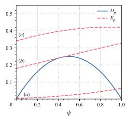
Figure 4. Example deposition and erosion closures, as functions of the solid fraction  $\psi$ . Steady flows occur where  $D_p$  and  $E_p$  intersect. There are three cases: (a) two steady states, one dilute and one concentrated (Fr = 0) 0.75); (b) a single steady state where  $E_p$  is tangent to  $D_p$  ( $Fr \approx 2.63$ ); (c) erosion always exceeds deposition (no steady states) (Fr = 3.25).
