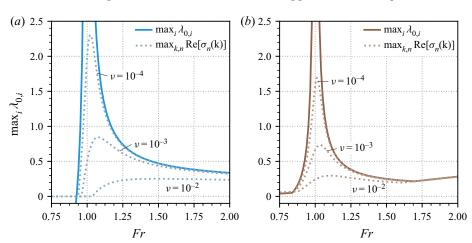
Figure 11. Effect of eddy viscosity size on the severity of morphodynamic instability. Solid curves show the maximum asymptotic growth rates for the unregularised system (as shown previously in figure 7), near the Fr = 1 singularity, for (a) dilute and (b) concentrated steady states. Dotted curves show the maximum growth rates over all wavenumbers and all four modes, for various  $\nu$ , as labelled.
