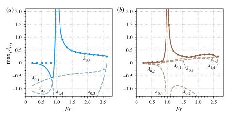
Figure 7. The maximum of the high-wavenumber asymptotic growth rates,  $\max_i \lambda_{0,i}$ , plotted with solid curves as a function of Fr, for the (a) dilute and (b) concentrated solution branches. With dashed lines we plot the individual  $\lambda_{0,i}(Fr)$  curves, as labelled for  $i=1,\ldots,4$ . Also plotted (filled circles) are the maximum growth rates of the corresponding solutions, over all wavenumbers, i.e.  $\max_{k,n} \text{Re}[\sigma_n(k)]$ .
