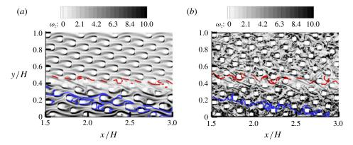
FIGURE 7. (Colour online) Distribution of the dimensionless vorticity magnitude  $\omega_z(H/u_b)$  within a high-Reynolds-number basal current propagating in a channel with  $\phi=12\,\%$  and D/H=0.05: (a)  $Re=15\,000$ ; (b)  $Re=150\,000$ . The dashed (red online) and the solid (blue online) lines show the C=0.05 and C=0.95 isocontours respectively. The distributions are shown in the region situated within the rectangle in figure 5(d).
