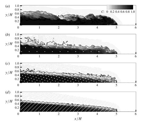
FIGURE 4. Distribution of concentration, C, within a high-Reynolds-number ( $Re = 15\,000$ ) bottom current propagating in a channel with (a)  $\phi = 0\,\%$ ; (b)  $\phi = 1.25\,\%$ , D/H = 0.032; (c)  $\phi = 5\,\%$ , D/H = 0.032; (d)  $\phi = 12\,\%$ , D/H = 0.032. Results are compared when  $x_f/H = 5$ . The solid line shows the C = 0.01 isocontour.
