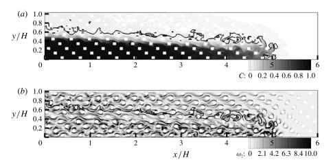
FIGURE 6. Distribution of concentration C (a) and dimensionless vorticity magnitude  $\omega_z(H/u_b)$  (b) within a high-Reynolds-number ( $Re=15\,000$ ) bottom current propagating in a channel with  $\phi=12\,\%$  containing large cylinders (D/H=0.07). The solid line shows the C=0.01 isocontour.
