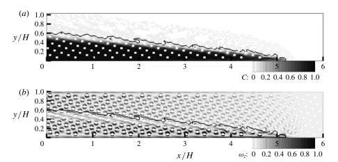
FIGURE 8. Distribution of concentration C (a) and dimensionless vorticity magnitude  $\omega_z(H/u_b)$  (b) within a low-Reynolds-number (Re = 375) bottom current propagating in a channel with  $\phi = 12\%$  and D/H = 0.032. The solid line shows the C = 0.01 isocontour.
