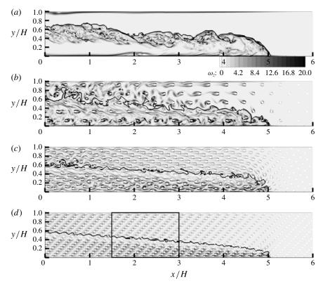
FIGURE 5. Distribution of dimensionless vorticity magnitude,  $\omega_z(H/u_b)$ , within a high-Reynolds-number ( $Re = 15\,000$ ) current propagating in a channel with (a)  $\phi = 0\,\%$ ; (b)  $\phi = 1.25\,\%$ , D/H = 0.032; (c)  $\phi = 5\,\%$ , D/H = 0.032; (d)  $\phi = 12\,\%$ , D/H = 0.032. Results are compared when  $x_f/H = 5$ . The solid line shows the C = 0.01 isocontour. The rectangle in frame (d) shows the region visualized in figure 7.
