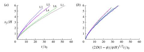
FIGURE 11. (Colour online) Temporal evolution of the front position,  $x_f/H$ , of the bottom current in the  $Re=15\,000$  simulations with  $\phi=5\,\%$ , D/H=0.032 (blue line L3),  $\phi=12\,\%$ , D/H=0.032 (dark grey line L1),  $\phi=12\,\%$ , D/H=0.05 (pink line L4),  $\phi=12\,\%$ , D/H=0.07 (dark blue line L5) and  $\phi=25\,\%$ , D/H=0.07 (green line L6). (a) Plotted against  $t/t_0$ ; (b) plotted against  $(2D(1-\phi)/\phi H)^{1/2}t/t_0$ .
