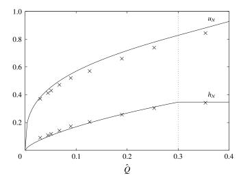
FIGURE 11. The dimensionless speed,  $u_N$ , and height,  $h_N$ , of the front as a function of the dimensionless flux per unit width,  $\hat{Q}$  calculated from the shallow layer with  $F_0 = 1$  (solid lines) and from the numerical simulations of Shringapure *et al.* (2013) (×). Also marked is the value of the flux,  $\hat{Q}_c$  at which the motion first becomes choked (dashed line).
