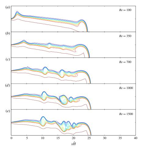
FIGURE 9. (Colour online) Contours of the dimensionless excess density field from the DNS at  $t = 20\hat{H}^{1/2}$  for source Froude number,  $F_0 = 1.2$ , and dimensionless flux,  $\hat{Q} = 0.42$ , at various Reynolds numbers. The ten contours in each panel correspond to values of  $\hat{\rho}$  from 0.1 to 1 with increments of 0.1.
