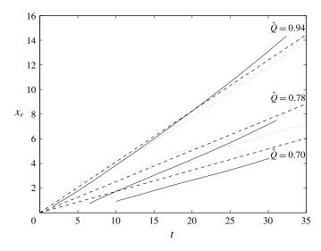
FIGURE 10. The position of the interface between the dense and less fluids at the upper boundary of the channel,  $x_r(t)$  as a function of time for cases in which the gravity current becomes channel filling close to the source from the DNS results at Re = 350 (solid lines), at Re = 1500 (dotted lines) and the shallow-layer modelling (dashed lines). The DNS results are curtailed when the basal front leaves the fluid domain.
