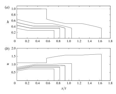
FIGURE 6. The height, h, and velocity, u as functions of x/t for two-layer currents that have lost their hyperbolic structure and transition to either channel-filling flows or to flows with critical control at the origin. In this plot,  $\hat{Q} = 0.2$ ,  $Q_{mc} = 0.3001$ , 0.4,  $Q_m = 0.5273$ , 1.1.
