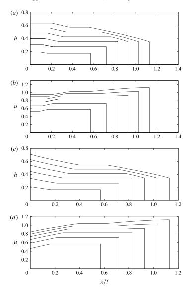
FIGURE 4. The height, h, and velocity, u, as functions of x/t for dimensionless fluxes  $\hat{Q} = 0.1, 0.2, 0.3, 0.4, 0.5, 0.6$  and (a,b)  $F_0 = 1.2$ , (c,d)  $F_0 = 1$ . Increasing values of  $\hat{Q}$  produce successively deeper and faster flowing currents in both (a,b) and (c,d).
