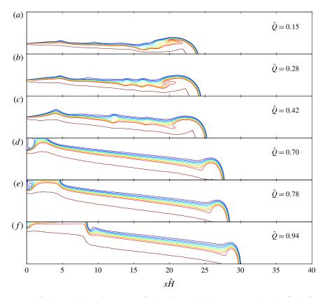
FIGURE 7. (Colour online) Contours of the dimensionless excess density field from the DNS at  $t=20\hat{H}^{1/2}$  for source Froude number,  $F_0=1.2$ , and various values of the dimensionless flux,  $\hat{Q}=0.15,\,0.28,\,0.42,\,0.70,\,0.78,\,0.94$ . The ten contours in each panel correspond to values of  $\hat{\rho}$  from 0.1 to 1 with increments of 0.1.
