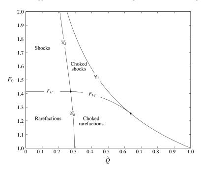
FIGURE 14. Regimes of Boussinesq solutions, classified in terms of the dimensionless flux per unit width,  $\hat{Q}$ , and the source Froude number,  $F_0$ , when circulation-based models are used for the conditions at the front and across bores.
