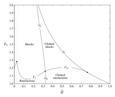
FIGURE 15. Regimes of Boussinesq solutions, classified in terms of the dimensionless flux per unit width,  $\hat{Q}$ , and the source Froude number,  $F_0$ , when an empirical model (Huppert & Simpson 1980) is used for the front condition.
