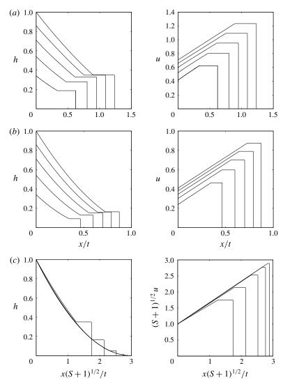
FIGURE 13. The height, h, and velocity, u as function of x/t for non-Boussinesq, supercritical source conditions  $F_0 = (1 + S)^{-1/2}$ ; (a) S = 1 and (b) S = 5 with  $\hat{Q} = n(1 + S)^{-1/2}/5$  (n = 1, 2, 3, 4, 5). Also plotted in (c) are the height and rescaled velocity fields as a functions of  $(S + 1)^{1/2}x/t$  for  $F_0 = \hat{Q} = (1 + S)^{-1/2}$ .
