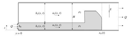
FIGURE 1. Configuration of the two-layer gravity current driven by a sustained source of dense fluid in a horizontal channel. In this sketch, the layer of dense fluid includes a bore connecting two regions within one of which the interface is of constant height and within the other it is thinning towards the front.
