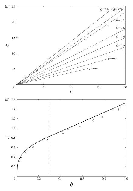
FIGURE 8. (a) The position of the front of the current,  $x_N(t)$ , as a function of time for each of the simulations with  $F_0 = 1.2$ ; and (b) the measured velocity of the current,  $u_N$ , as a function of the dimensionless flux,  $\hat{Q}$  at Re = 350 (O) and Re = 1500 (×). Also plotted are the predictions from the shallow-layer analysis (solid line) and the asymptotic result when  $\hat{Q} \ll 1$  (dotted line) and  $\hat{Q} = 0.2938$  at which value the flow becomes choked.
