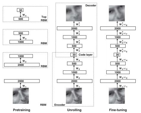
**Fig. 1.** Pretraining consists of learning a stack of restricted Boltzmann machines (RBMs), each having only one layer of feature detectors. The learned feature activations of one RBM are used as the "data" for training the next RBM in the stack. After the pretraining, the RBMs are "unrolled" to create a deep autoencoder, which is then fine-tuned using backpropagation of error derivatives.
