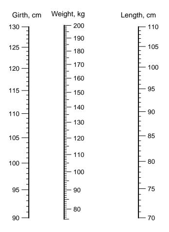
Figure 6: Nomogram for Kenyan donkeys with BCS = 3 and Age = >5. To predict Weight, join the Girth and Length values with a straight line.
