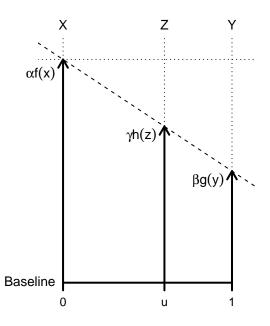
Figure 2: Geometry of a parallel-scale nomogram, after Fig. 2 in Doerfler (2009).
