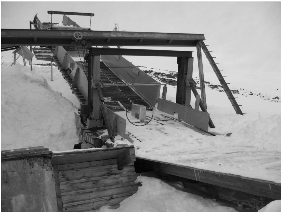
Figure 4: Photograph of the SLF snow-chute at Weissfluhjoch, in Davos, Switzerland. The circle in the centre of the picture indicates the half-wedge containing the optical sensor array. Photograph: M. Schaefer, SLF.
