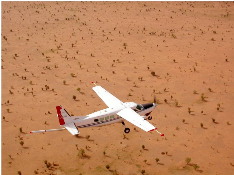
Survey aircraft ( \approx 50\text{ms}^{-1} , \approx 200\text{m} above ground)
